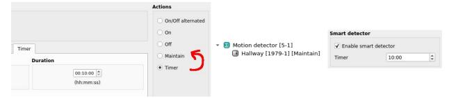
Now, motion detector will not send new motion detection over the bus until end of timer.
