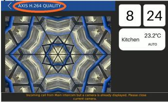
A communication with DoorBird® door station can be established directly from the DTSC05 using cameras menu.
