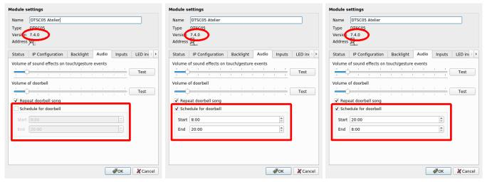
DTSC05 can ring at any DTSC05 can only ring DTSC05 can only ring time between 8:00 and 22:00 between 22:00 and 8:00 (night)
