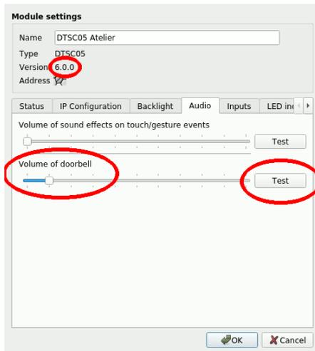
already been flashed in version 6.0.0 or newer, the **Test** button can be used to test the volume directly on the DTSC05. **Attention:** maximum volume is very loud. Use it carefully.
