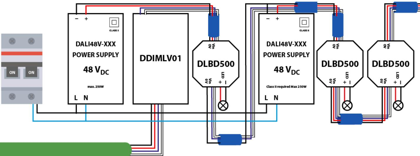
The number of power supplies required is calculated according to the maximum power of the power supplies and the total power of the lamps.
