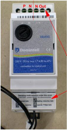
The DD400L is a dimmer module, intended to be connected within a Domintell system to a DDIM01 module, and designed for cabinet installation on Din rail in electrical networks 230V AC 50 Hz.
