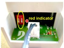
Selection is done manually with the DIP switch located inside the DD400L, under the plastic cover (down) protecting the DDIM01 connection. Use a small flat blade screwdriver to open, after having fully disconnected the unit from the electrical power network. After reconnection, the selection is confirmed by the number of flashes of a red indicator. Then re-install the cover
