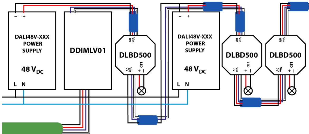
The number of power supplies required is calculated according to the maximum power of the power supplies and the total power of the lamps.
