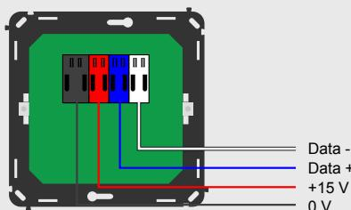
Domintell – 2 keys push-button, with RGBW LEDs and T ° probe
